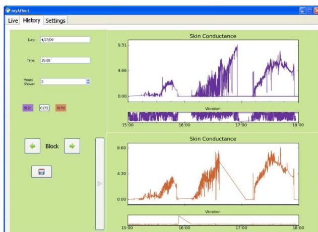
Figure 3.1 Initial Interface for Measuring Children during Occupational Therapy. Orange and Purple are skin conductance responses from two different legs.
